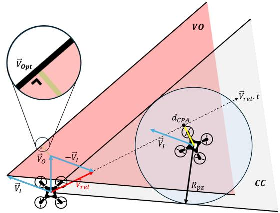
Figure 2: Illustration of Velocity Obstacle algorithm. The red-shaded area is a set of velocity that will lead to a loss of separation. Projecting the current ownship velocity to the nearest edge resolves the conflict with the least velocity change.
