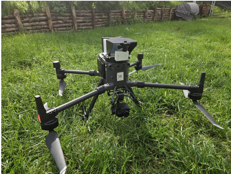
Figure 4-12 The device for GA and the Action Cam onboard of Drone 1
