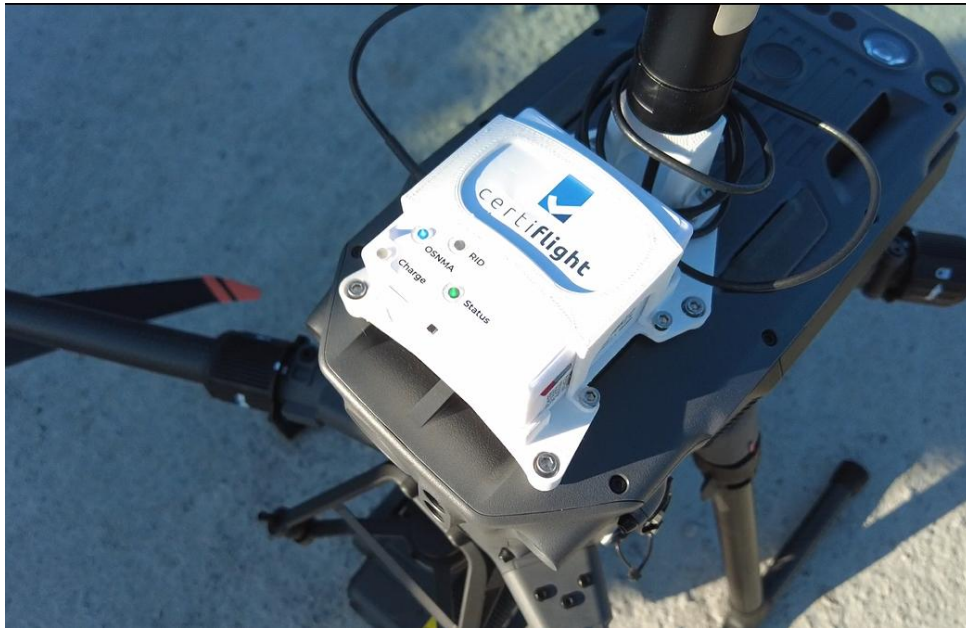
Figure 4-1 Device for UAS installed on the drone
