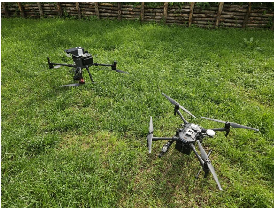
Figure 4-13 The drones used for the test with the devices onboard
