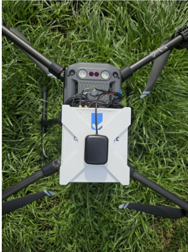
Figure 4-6 Device for GA installed on the drone
