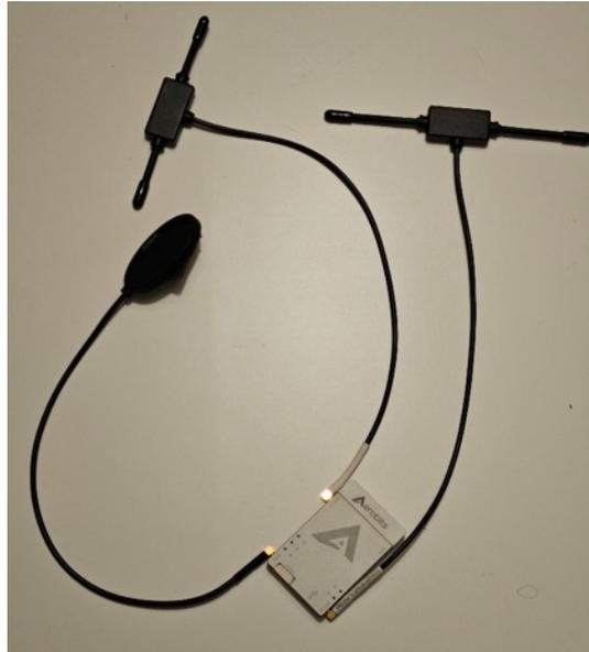
Figure 4-46 Aerobits HOD FLARM transceiver
