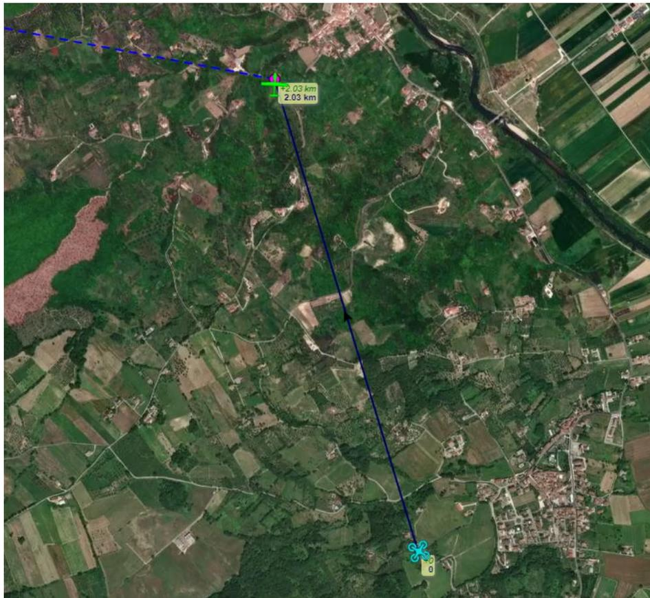
Figure 4-59 Maximum transmission distance shown on the ground antenna software
