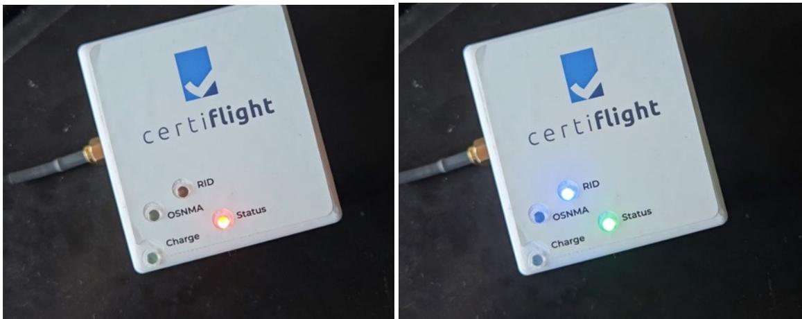
Figure 4-14 Low battery notification with STATUS LED red and green flashing
