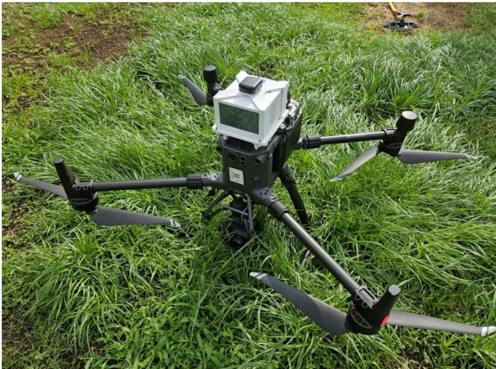
Figure 4-50 The device for GA installed on DJI M300
