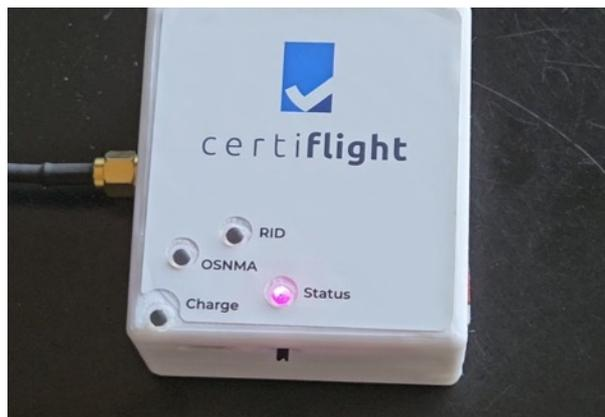
Figure 4-19 STATUS LED notifies fully loaded micro-SD error (solid PURPLE)
