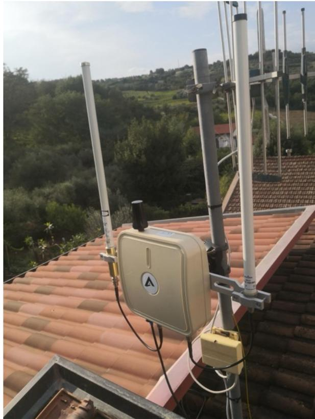
Figure 4-51 Aerobits FLARM on-ground station
