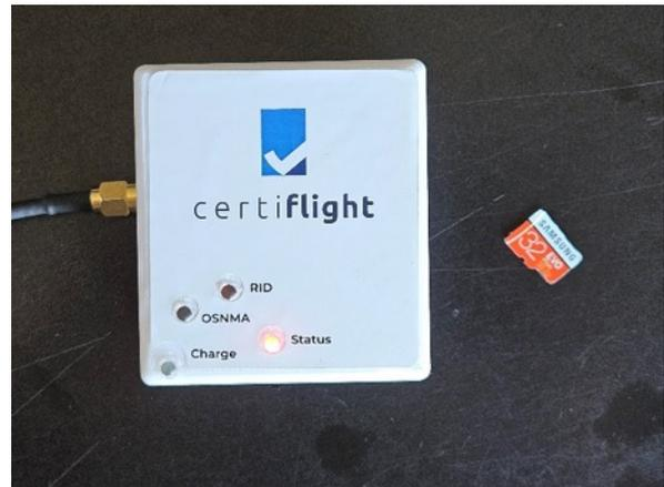
Figure 4-17 STATUS LED notifies missing micro-SD error (solid RED)
