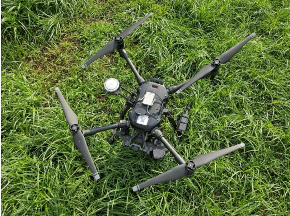
Figure 4-53 The second drone DJI M200 with FLARM transceiver
