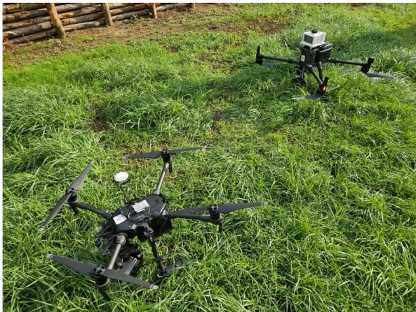
Figure 4-54 The drones used for FLARM reception test
