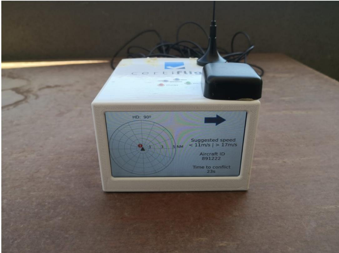
Figure 4-45 Warning message displayed on the device
