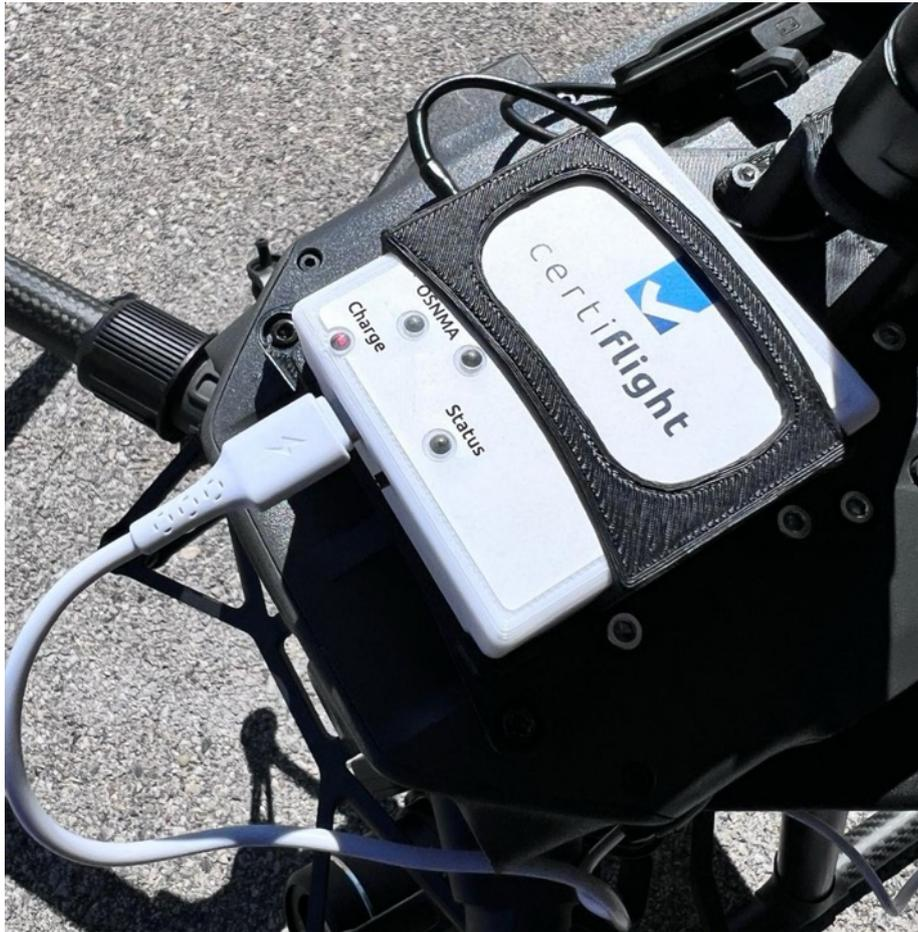
Figure 4-15 The UTM installed on the drone while charging
