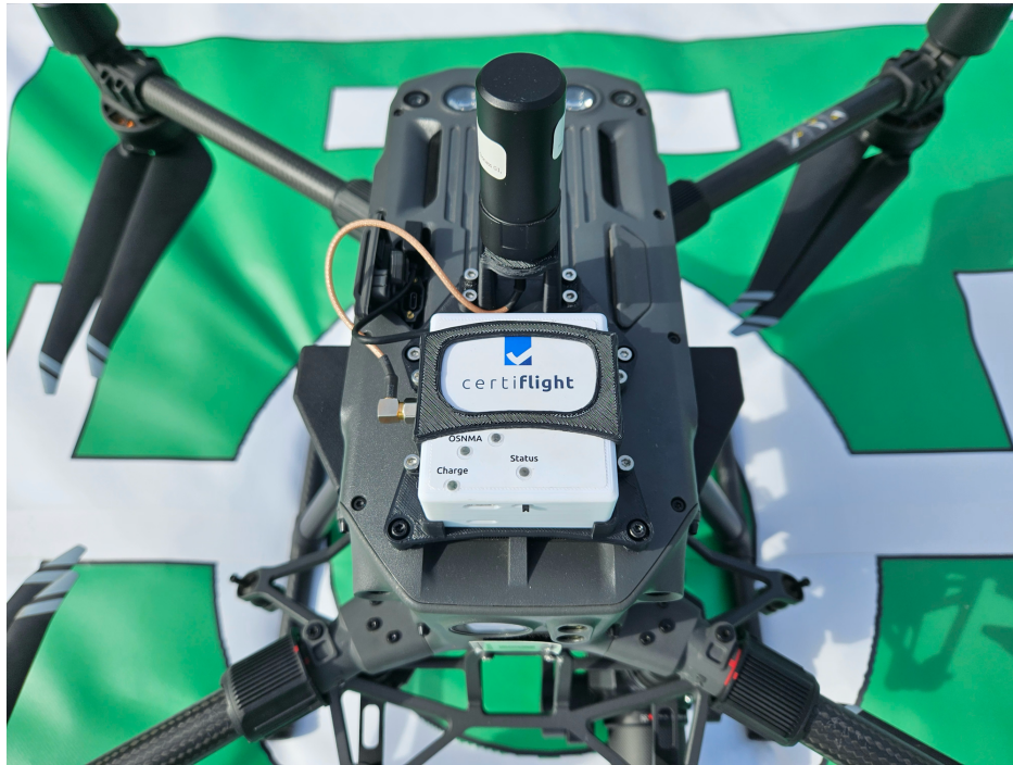
Figure 6-2 Device mounted on DJI M300
